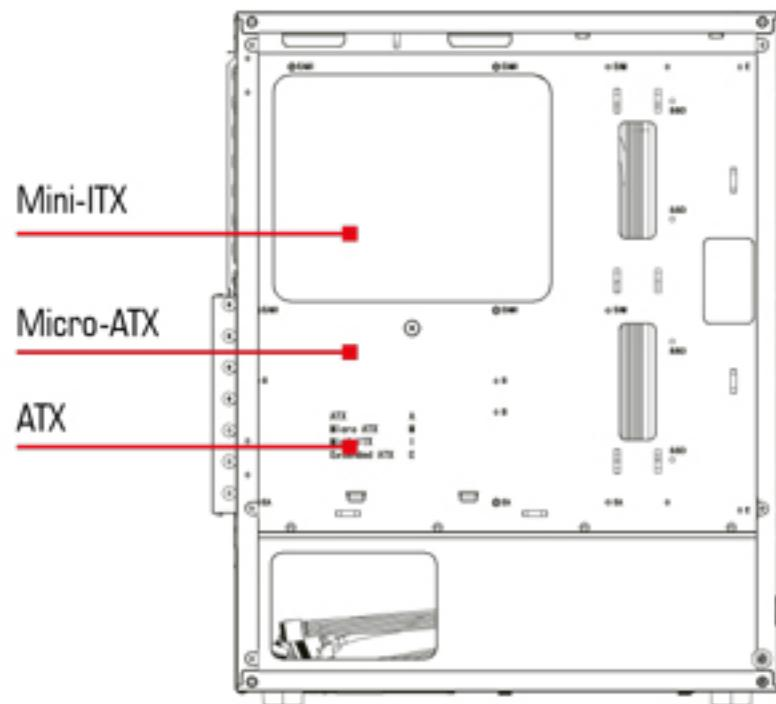
Motherboard Support: ATX / Micro-ATX / Mini-ITX
