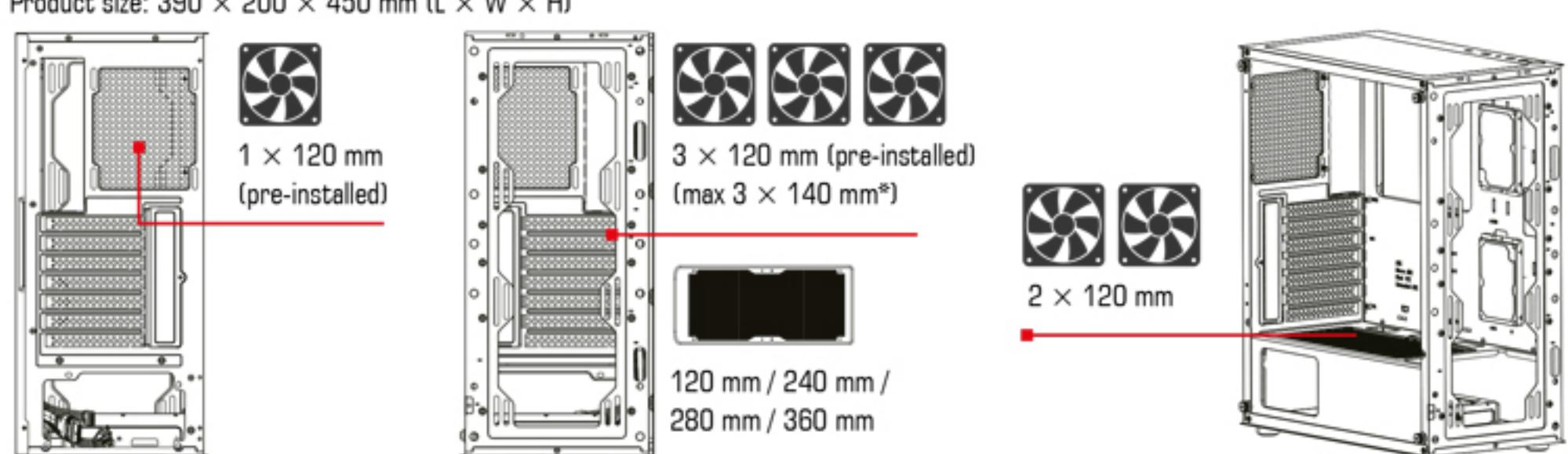
\* Installing 3 x 140 mm fans on the front of the case is possible only from the inside of the case. Four 31 mm screws (included) are needed for 2 top and 2 bottom holes.
