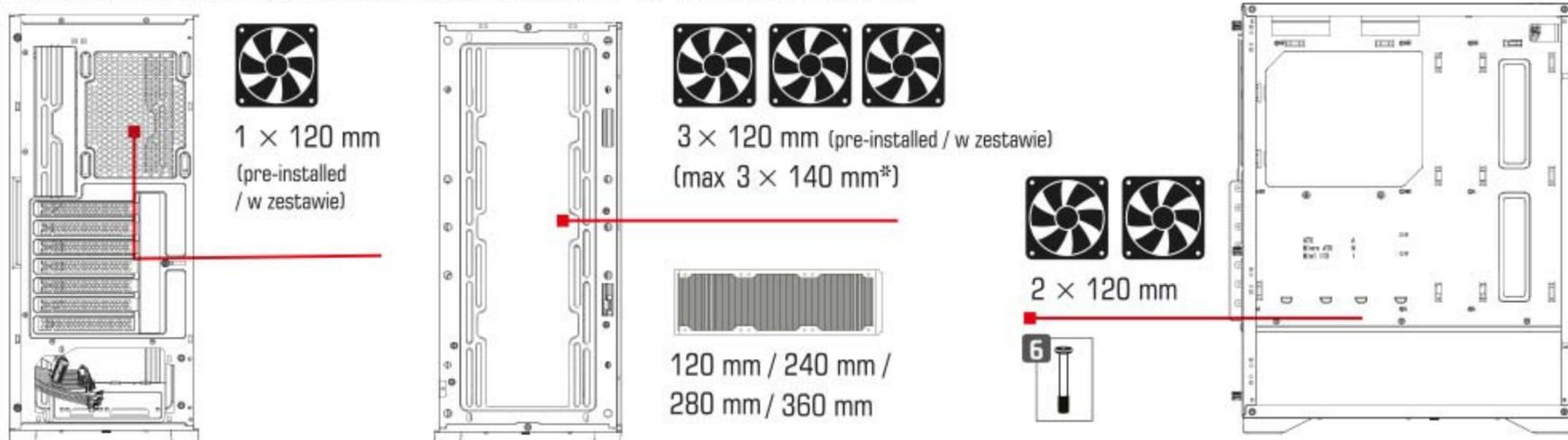
\* Installing 3 x 140 mm fans on the front of the case is possible only from the inside of the case.
