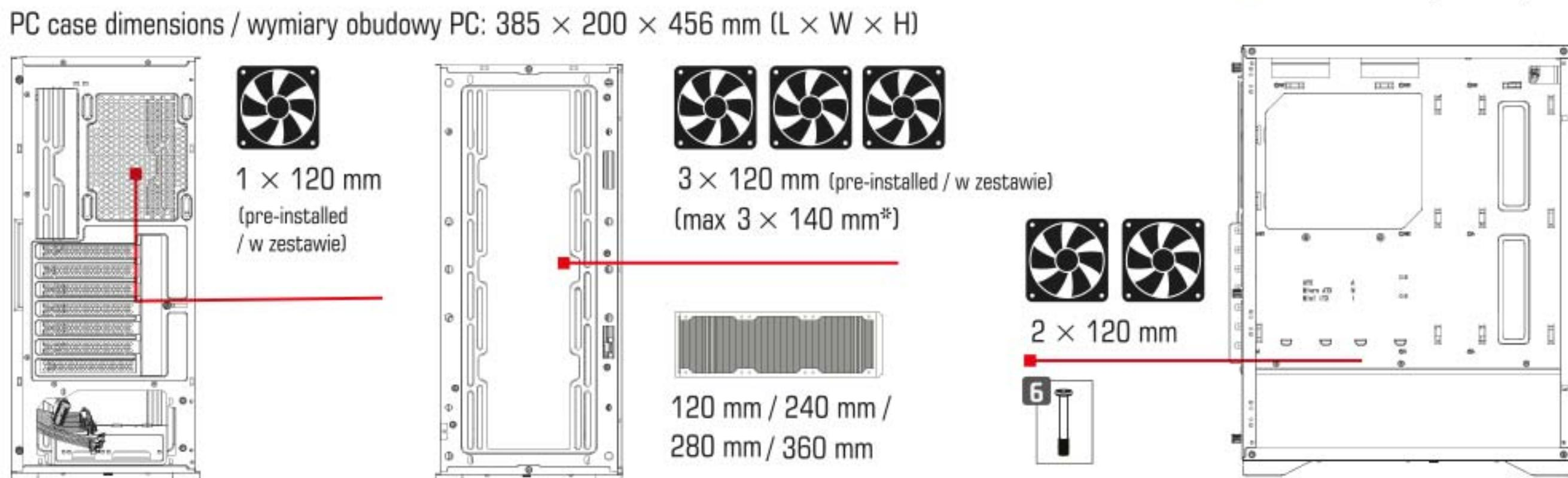
\* Installing 3 x 140 mm fans on the front of the case is possible only from the inside of the case.
